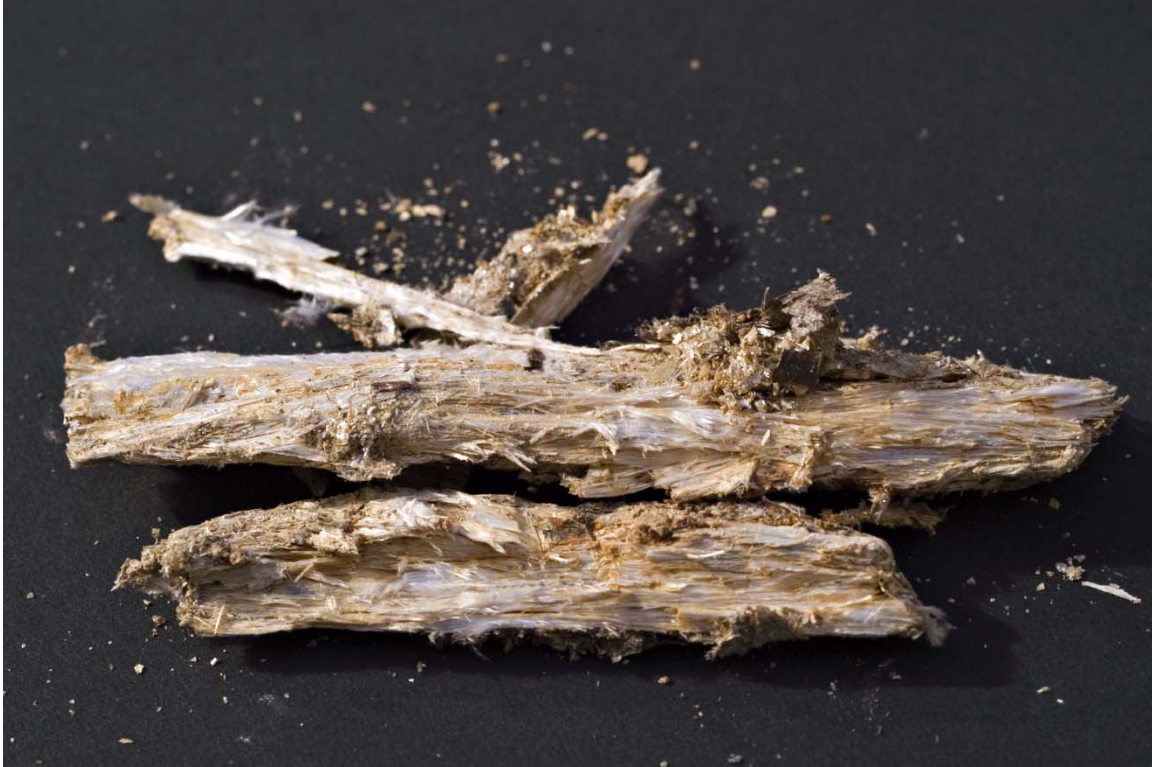
Some of the anthophyllite-rich rock is extremely friable and is easily airborne when dry and disturbed by physical abrasion.
